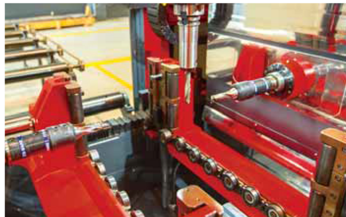
Through 3 independent spindle units on 3 ADM model, the profile can be drilled from 3 sides at the same time.
