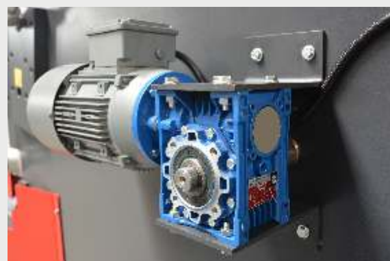
Motorized Blade Gap Adjustment with CNC Controller
