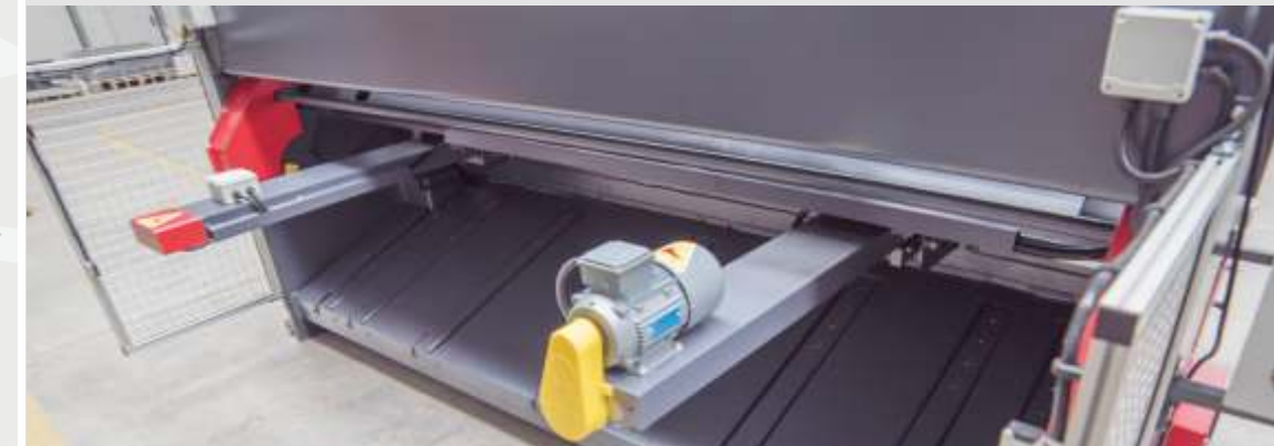
Motorized Back Gauge has \pm 0,1\text{mm} Accuracy
